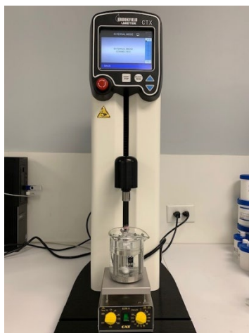
Figure 1. CTX Texture Analyzer (Ametek Brookfield, USA) equipped with a load cell of 1.5 Kg.
