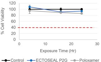
The toxic exposure time ( $ET_{50}$ ) is the time when cell viability is reduced to 50%, which is represented by a red dashed line in the Figure above. The general guideline for correlation of *in vitro* and *in vivo* results states that products with an  $ET_{50}$  of 24 hours are expected to be non-irritant. According to the results obtained, the  $ET_{50}$  of both EctoSeal P2G and Poloxamer is superior to 24 hours and, therefore, both products have a good safety and toxicological profile.
