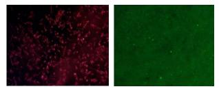
**Figure 3.** Representative images of stained biofilms using an inverted fluorescent microscope: red staining (10x magnification) indicates dead cells whereas green staining (4x magnification) indicates live cells.
